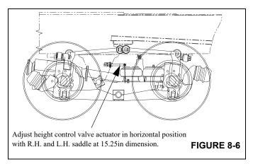
Adjust rod to achieve proper ride height setting (Figure 8-7) and torque P-clamp on P-boot to 10 - 15 in lbs.
