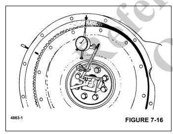
4. Secure a dial indicator to the crankshaft. With the gauge finger against the housing pilot, rotate the crankshaft. Use a marker or soapstone to mark the high and low points.
