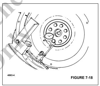
**6.** Move the gauge finger to contact the pilot bearing bore surface. Again, rotate the flywheel.
