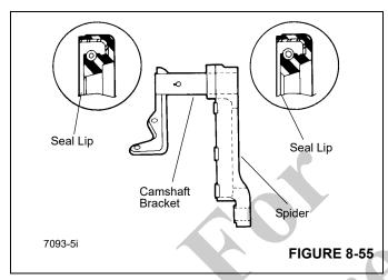
4. Put the cam head thrust washer on the camshaft. Apply O-617-A or B chassis grease to the camshaft bushings or needle bearings and to the camshaft journals. Install the camshaft through the spider and bracket so that the camshaft turns freely.
