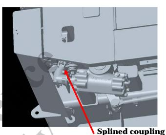
For minor/fine adjustment of the steering wheel loosen the clamp bolts and rotate the steering link to orient the steering wheel straight ahead. Apply Loctite 243 to clamp bolts and re-torque to 50-60 lbf\*ft. (68-81 N\*m).
