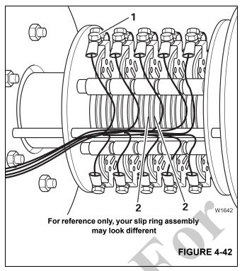
Remove visible dirt on the slip rings (2), (Figure 4-42) with a clean, lint-free cloth.
