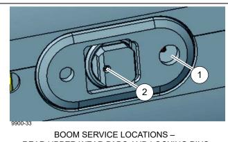
REAR UPPER WEAR PADS AND LOCKING PINS
