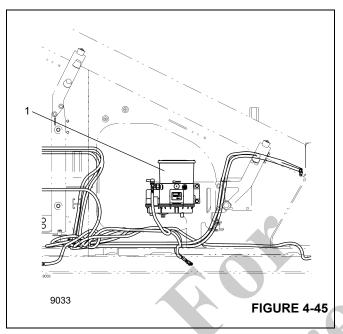
The grease container (1), (Figure 4-45) is located on the right side of the turntable above the storage compartment.
