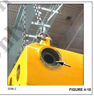
4. Lubricate the pivot bushings in the turntable.
