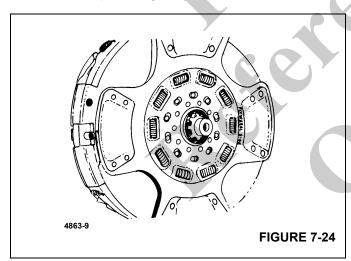
**6.** Install the front disc on the aligning tool with the side stamped "flywheel" facing the engine.
