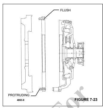
**5.** Positive Separator (Roll) pins should be flush on the clutch side, protruding on flywheel side.
