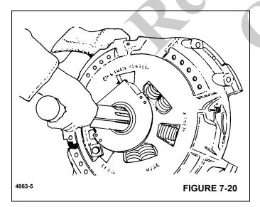
**3.** Put the rear driven disc on the aligning tool with the side stamped "pressure plate" facing the pressure plate.
