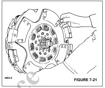
**4.** Place the intermediate plate in the clutch cover and align the driving lugs of the plate with the slots provided.
