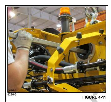
Reach in access hole at top of boom, install pins on stop plates already installed on back of mounting pins (Figure 4-12).
