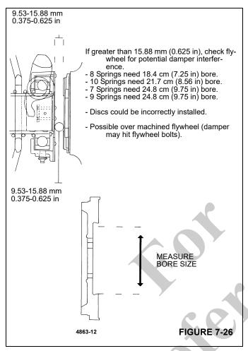
If greater than 15.88 mm (0.625 in) check possible disc to flywheel bore interference.
