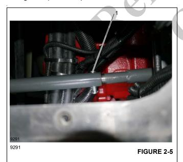
3. Separate the shift rod to gain access to pump no. 1.
