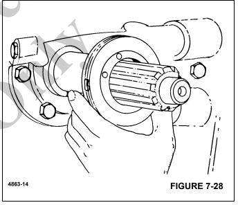
If a clutch brake is used, be sure to install it on the input shaft of the transmission at this time.
