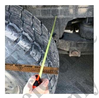
Adjust <u>front steer axle</u> drag link until front and rear measurements are equal. Apply Loctite 243 to clamp bolts and re-torque to 50-60 lbf\*ft. (68-81 N\*m).
