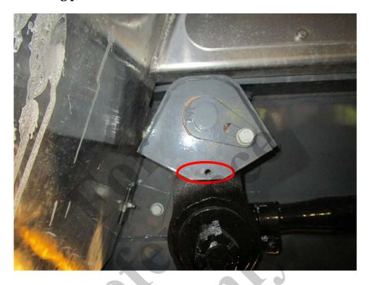
• Adjust the intermediate drag link to center the rear relay arm and pin it with a Ø 21/64 in. (0.8 mm) rig pin or drill bit. Apply Loctite 243 to clamp bolts and retorque to 110-130 lbf\*ft. (149-176 N\*m).
