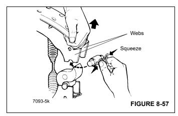
**4.** Push the retainer into the brake shoe until its ears lock into the holes in the shoe webs (Figure 8-57).
