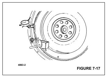
Move the gauge finger to contact the face of the engine flywheel housing.
